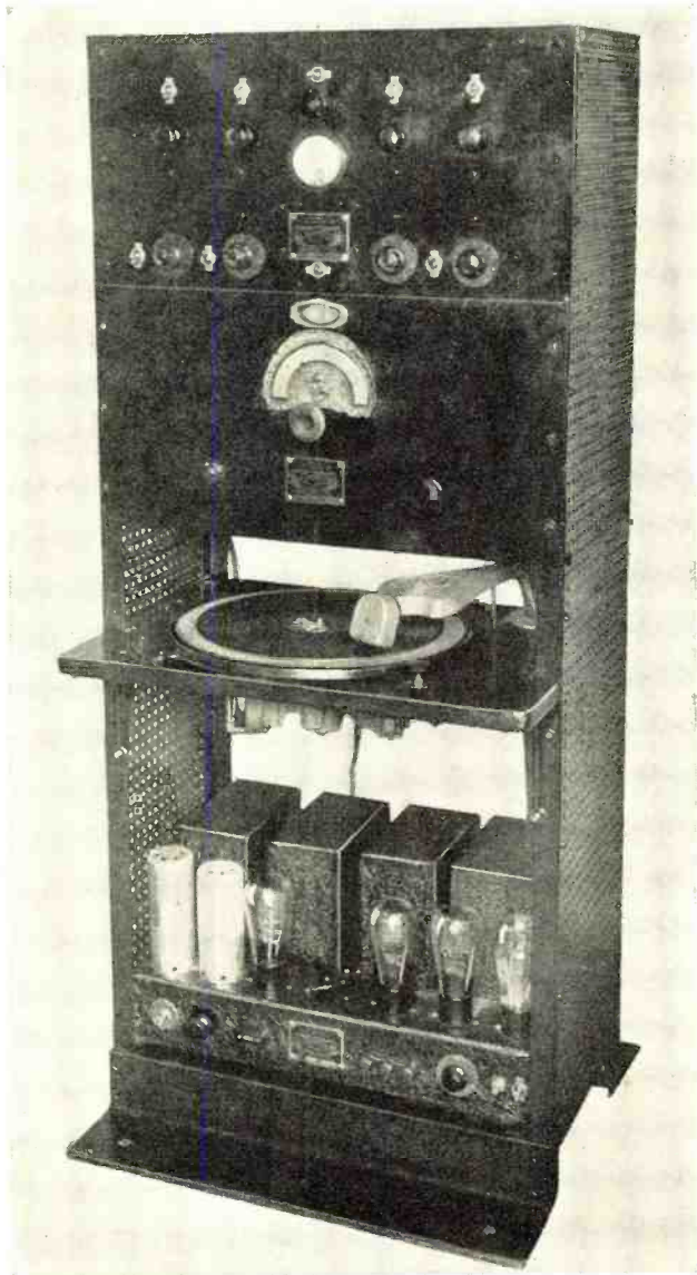
COMPLETE P.A. SYSTEM
