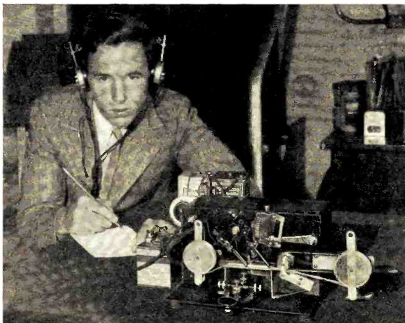
The master teleplex reproduces the message exactly as it was sent, but the speed can be adjusted
