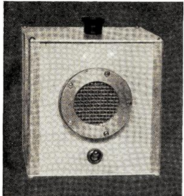
THE ABSORPTION MICROPHONE UNIT The standard 4½-inch aluminum box shield houses the head amplifier. The microphone mounted on the face is the Argabrite condenser microphone, constructional details on which were given in the April issue
