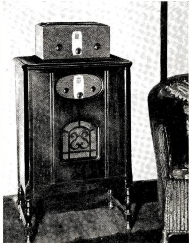
The new converter mounted atop a regular broadcast set and extending its range down to 15 meters when the switch on the converter is thrown to the short-wave position. Reversing this switch connects the antenna direct to the broadcast receiver
