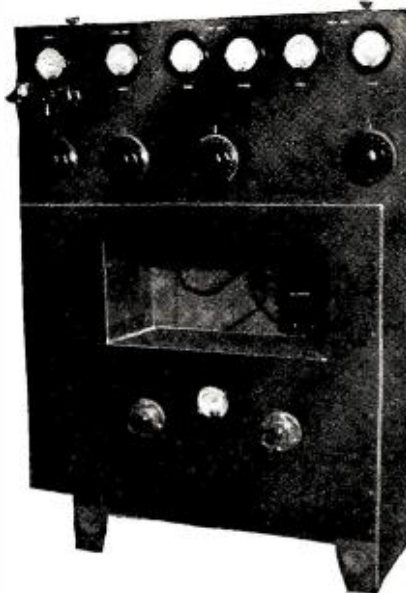
Front view of transmitter and below it the cabinet containing the relays (behind window), filament transformers and low-voltage plate supply. The filament rheostats and filament voltmeter are seen on the lower panel
