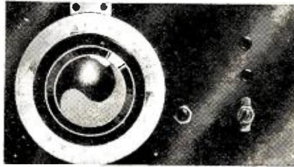
Figure 4. Front view of the serviceman's vacuum tube voltmeter. A direct reading calibration contributes much to the speed, accuracy and general utility of the instrument
