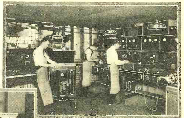
Radio Studios, Inc., New Rochelle, N. Y., submitted the photo shown above. The main test panel includes a complete set and tube tester, a high and low-resistance bridge, a 175 and 180 kc. oscillator. The small panel includes a continuity test, a milliammeter and a voltmeter connected to pin jacks. Both boards are wired with battery set voltages
