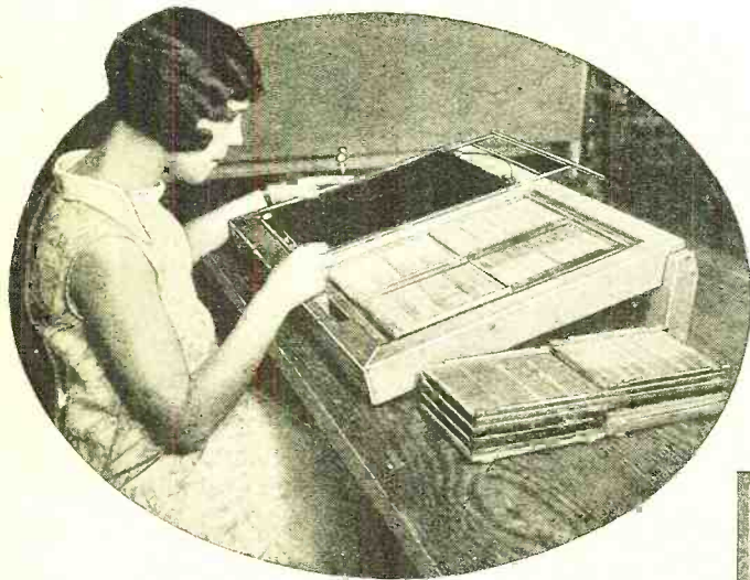
(Above) How X-ray photographs eliminate defective cathodes. A bright light below the film enables the inspector to locate defective cathodes in the film. The inspector places a pointer over the photograph of the defective cathode and a clever pantograph arrangement causes a similar pointer to come to rest directly over the defective cathode itself
