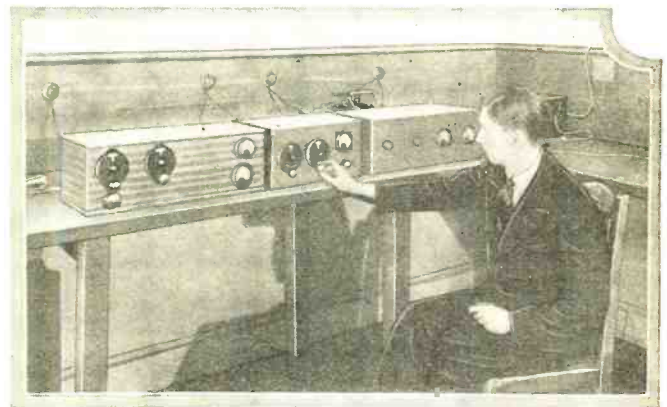
Mr. Percy Harris, well-known British receiver designer, operating the main tuning control of the laboratory model Stenode Radiostat
