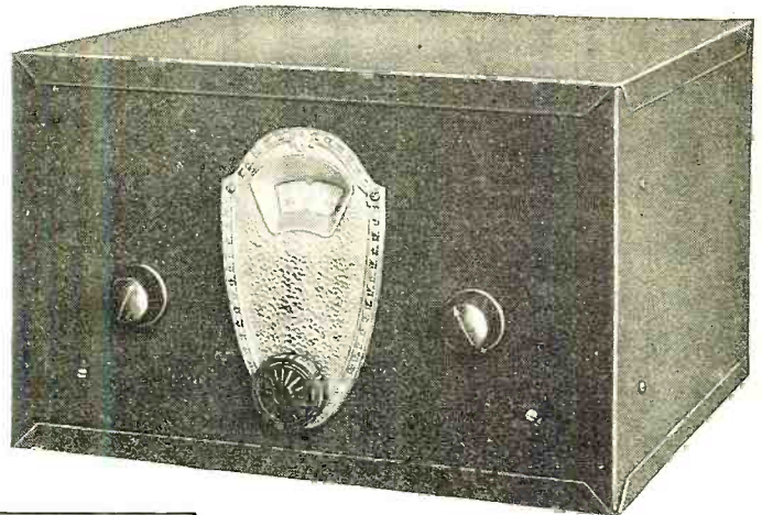
Fig. 4. A front view of a short-wave superheterodyne converter, attachable to any standard broadcast receiver
