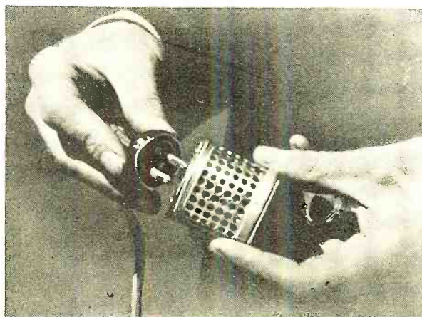
A plug-in type of line voltage regulator. It is merely necessary to plug in the plug from the cord on the receiver and then plug in the regulator to a convenient wall socket to put it into service
