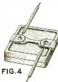
Fig. 4. Bend back the lugs on the fixed condensers and make the connections as shown
