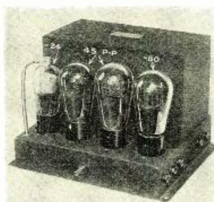
The push-pull amplifier in outward appearance is much like the conventional single output tube amplifier. In the above, two -45's are used in push-pull
