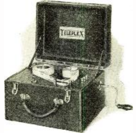
One type of a code learning device. A spring motor equipped with a regulator permits the operator to adjust the transmitting speed
