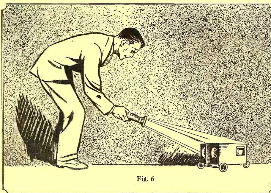
"The Electric Dog," invented by John Hays Hammond, Jr., some years ago, is an ingenious toy; but the principle may be applied to practical purposes. The movements of the little self-propelled box are guided toward or away from the light, as desired by the operator.
