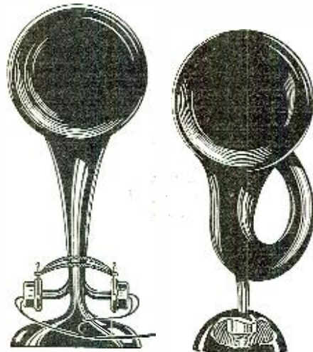
Fig. 3 (left). An early speaker which employed a pair of phones as a driving unit. Fig. 4 (right). Another early speaker, with phone unit mounted in base.
