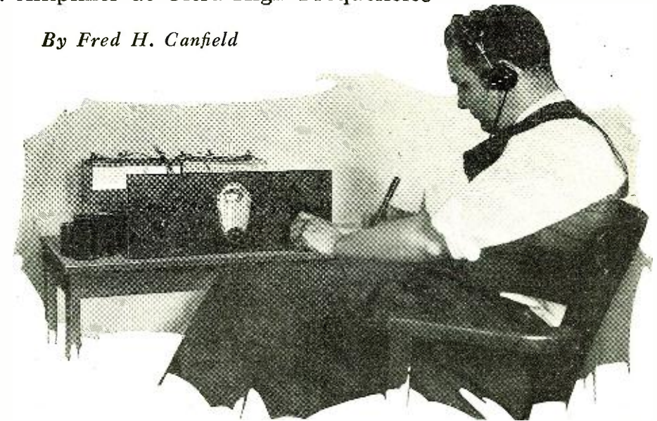
Fig. A. This picture, taken in RADIO NEWS Laboratories while testing the Screen-Grid Short-Wave Receiver, clearly shows the neat, unencumbered appearance of the front panel. The coils for other wavebands are at the left.
