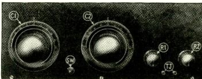
At the right is shown the front panel view of the 4-tube Knickerbocker receiver. The dials, C1 and C2, control the variable condensers having similar designations; R1 and R2, filament rheostat controls; SW, filament switch; and TJ, tip jacks for loud speaker.
