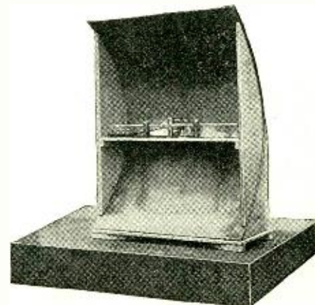
Marconi's early model receiver for focusing the signals from beam transmission, designed by him in 1895.
