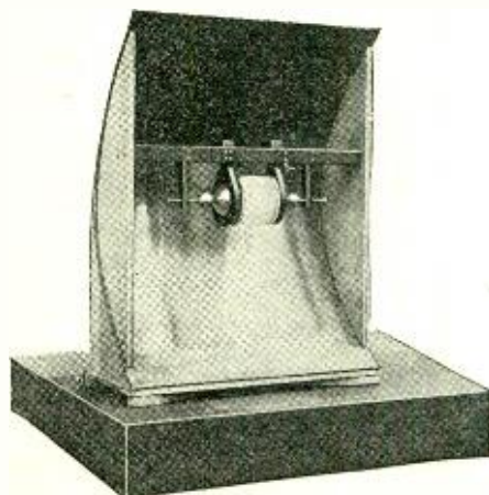
This picture shows a very early model transmitter, invented by Marconi for short-wave beam-radio work.
