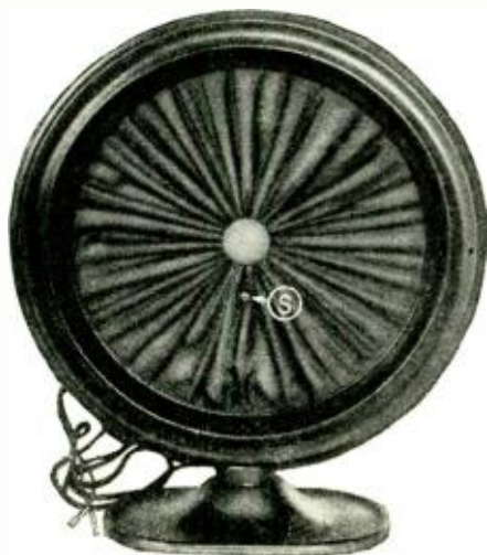
This is the actual front of the cone speaker. The letter S indicates the adjusting screw.
