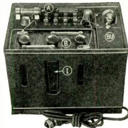
The "A-B" power unit with the top removed. A is the rectifier for the battery charger; B, the six-volt storage battery; BU, the "B" supply section; I, glass side of the battery jar through which the indicator balls may be viewed.
