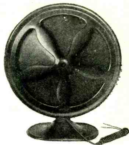
Left: The back of the cone speaker, with the silk cover removed to show the position of the drive-unit on the upright section of the frame. Right: The front of the same speaker.
