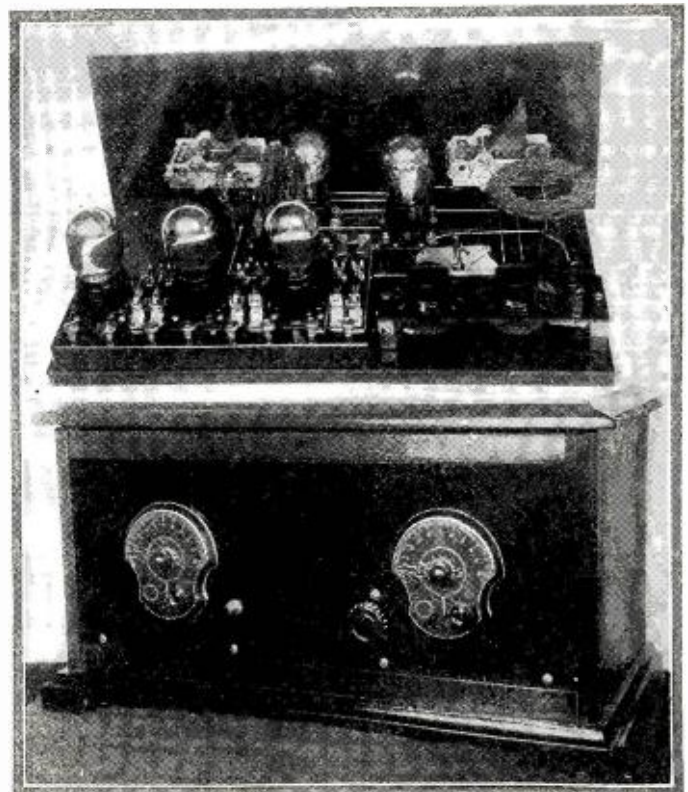
Above is reproduced a photograph from the rear of the interior of the Parlor Music Maker. The two variable condensers employed are the straight-line frequency type, to insure ease in tuning. The resistance-coupled audio frequency amplifier is shown on the left of the baseboard. Below is shown the complete receiver in its cabinet, fit for any parlor.
