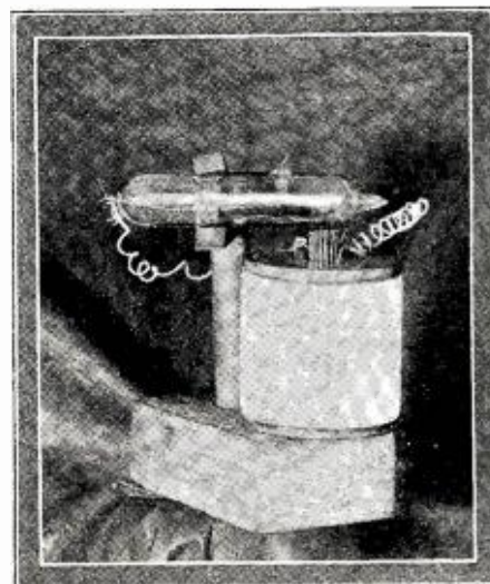
The actual original model of Moore's "Turn-Down" electric lamp. A vibratory contact inside the glass is operated by an external magnet.
