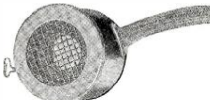
The condenser microphone, used in Germany, which consists of two metal discs 1/1000 of an inch apart, one of which is free to vibrate, setting up changes of potential in the circuit.
