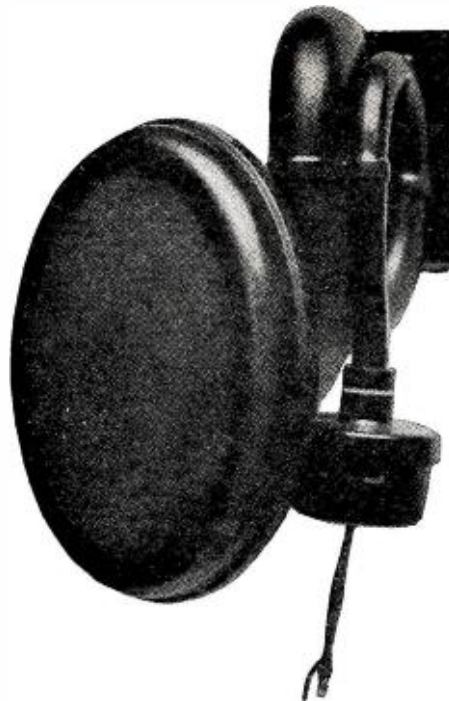
Fig. 2. An older type of loud speaker horn which employed curved tubing to obtain an effective long column of air.
