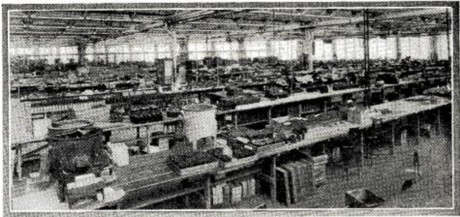
One of the coil departments. Note the vat of impregnating compound, and the various jigs for use in completing the coils, before they are sent to the assembling departments.
