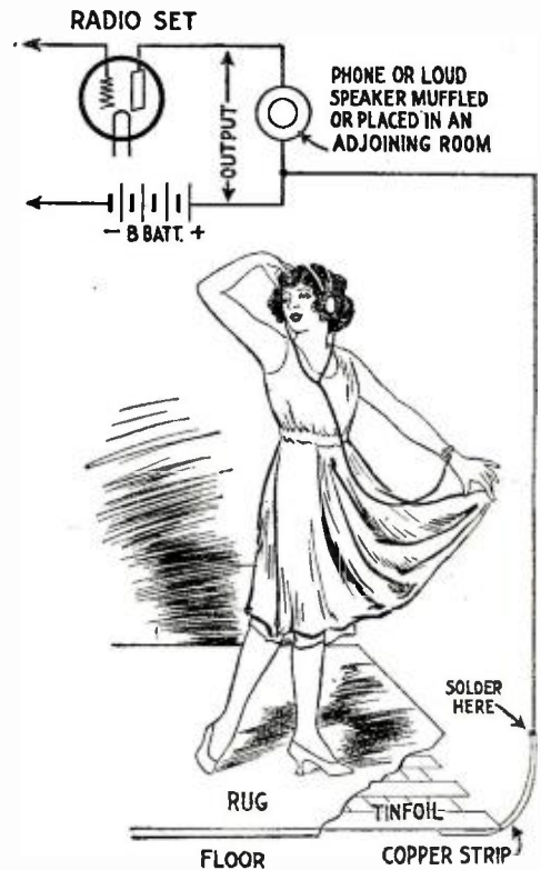
Fig. 3. Electrical connections showing how tinfoil under the rug is connected with the output of a multi-tube radio set. With some sets it is necessary also to ground one connection: the phone may be muffled, or the cap and diaphragm taken off, as shown in Fig. 4.
