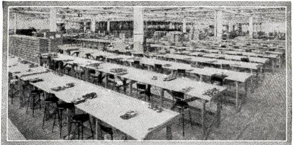
An assembling room, showing the trays in which the unit parts are supplied, and the finished instruments to the right of each worker's place.
