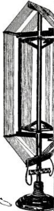
Fig. 2162-A. An audio frequency oscillator, involving the use of a Neon tube.
