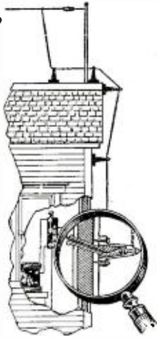
Note—that the pedestal is hollow and may be used to conceal the end of the wall tube.
