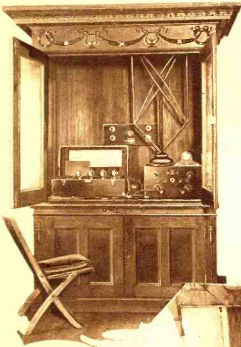
MAIN RADIO EQUIPMENT AT SING SING. The receiver, on the left side of the cabinet, remains in the cabinet and the amplifier is carried to the different parts of the prison when it is desired to entertain the prisoners. © Kadel & Herbert.
