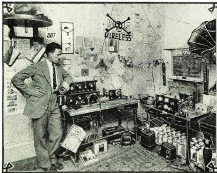
On the left side of the "shack" is the author's receiving set and on the table on the right side of the photograph is the transmitting station. The underground antenna is used for both receiving and transmitting.
