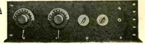
R. E. Lacault, A.M. I.R.E., the well-known radio engineer, designed and developed the "Ultradyné" shown above. It is a six tube receiver with splendid power, easy to wire and construct. The latest in 1925 radio models.
