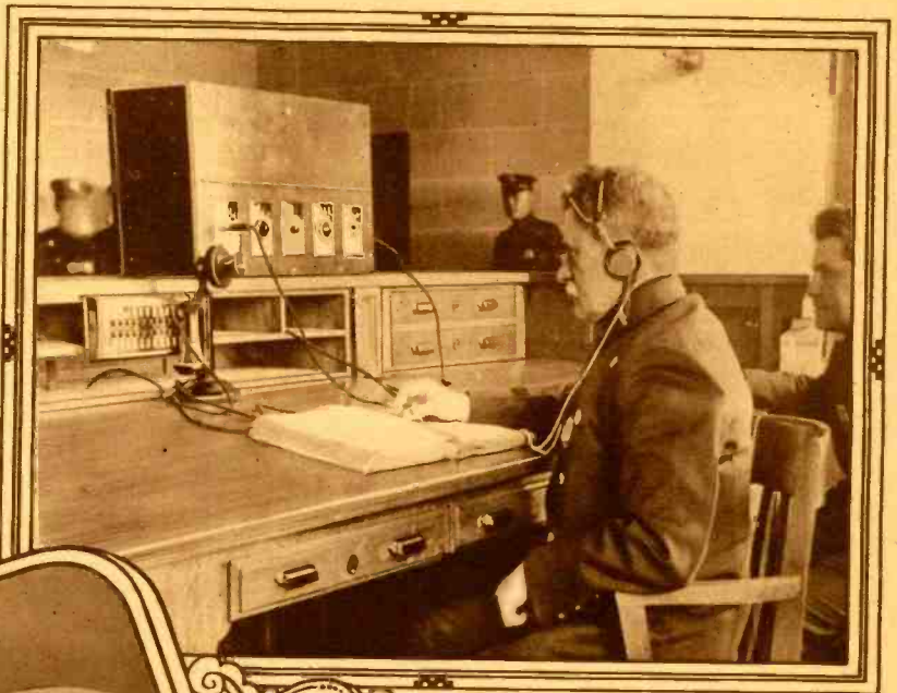
IN THE STATION HOUSE. When a station house is signaled, a light flashes and a bell rings in the receiving set, which is tuned only to the wave-length of WNYC. © Fotograms.
