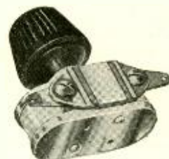
Fig. 6. A carbon pile grid leak of this nature allows the adjustment of the resistance to be made to a very fine degree.
