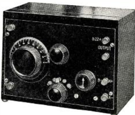
Fig. 3. An excellent type of compact single tube receiving set for use with headphones.
