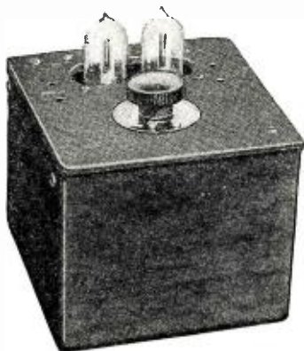
Fig. 7. Above is shown a two-tube push-pull amplifier to be used with the set shown in Fig. 6 or any other one- or two-tube receiving set.
