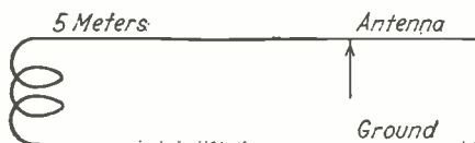
The arrow shows the position at which the Tungar bulb is placed in the antenna circuit of the 2-meter transmitter.
