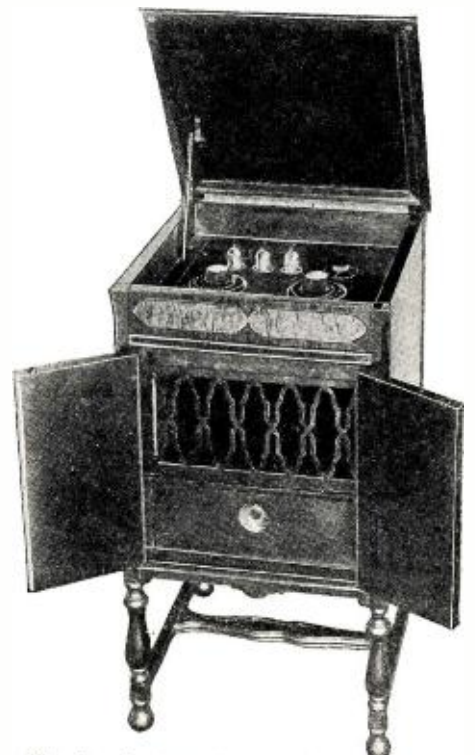
Fig. 10. A three tube receiving set using a reflex circuit incorporated in a handsome cabinet.
