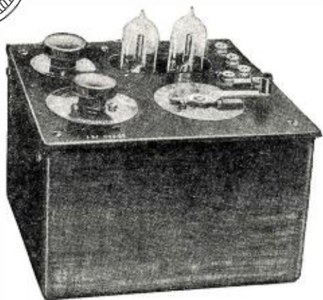
Fig. 6. Above is shown a two-tube receiving set which is very simple to tune and which gives good volume on local stations.
