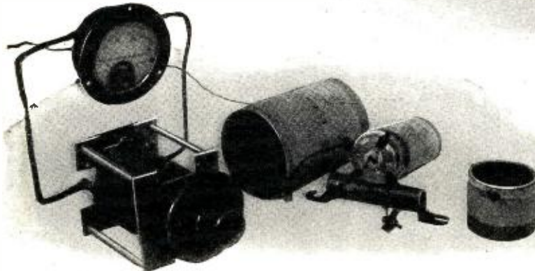
Fig. 4. Another view of the tube with its base removed, resting on the grid leak. Note the R.F. chokes to either side of the tube. The wavemeter is in the foreground.
