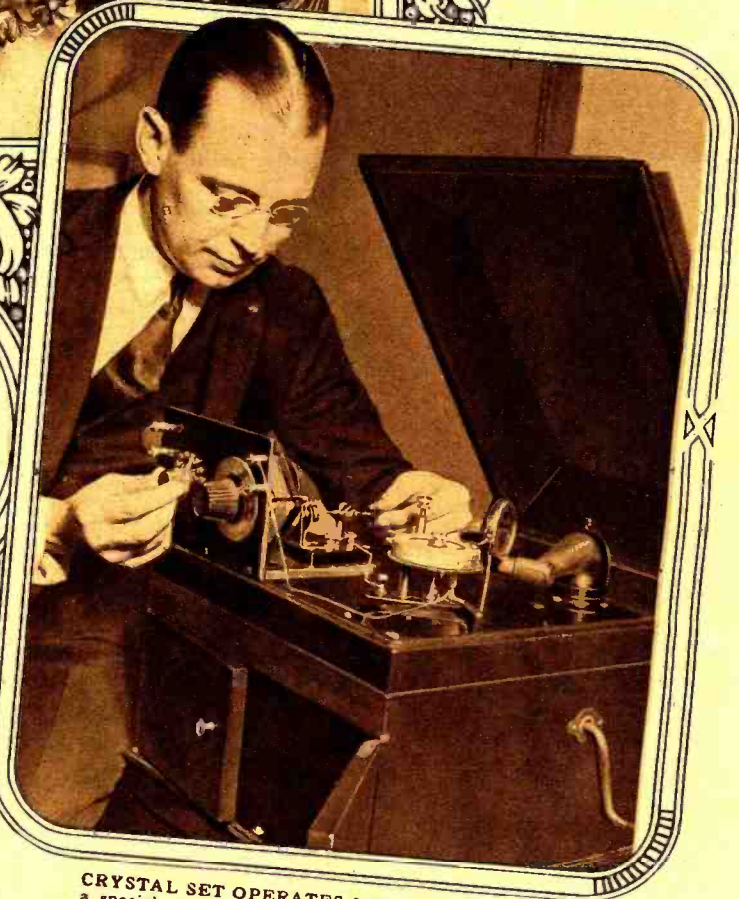
JUST A HANDFUL. This miniature single tube regenerative set of unusual construction works as well as its big brothers. Note the scale engraved on the foremost rotary plate of the variable condenser. The pointer is stationary. © Kadel & Herbert
