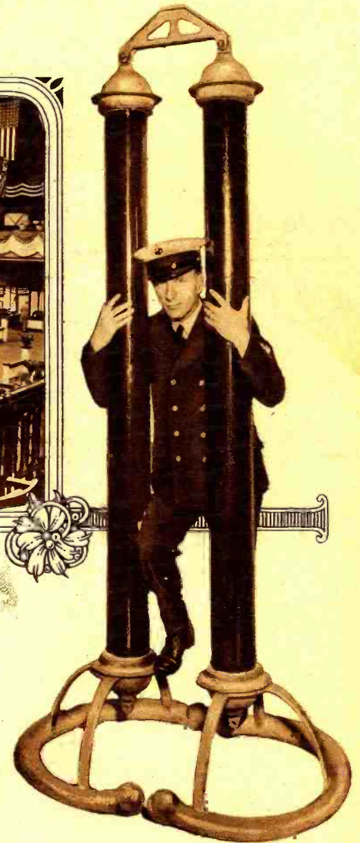
THE LARGEST RADIO INSULATOR in the world; one of the many insulators designed particularly for the high powered shore radio stations of the U. S. Navy, exhibited at the Radio World's Fair. How about a couple of these for your aerial? © Kadel & Herbert.
