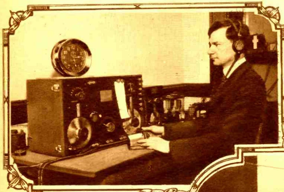
Left: Here is Paul Sollenburger, the man who attends to the transmission of the time signals from the U. S. Observatory at Washington, D. C. The signals are relayed from Washington by wire to the transmitting station, NAA at Arlington, Va., which works on a wave-length of 2,650 meters. This is a very powerful station and the time signals transmitted at noon and at 10 P.M. are heard by ships in both the Atlantic and Pacific oceans. No matter where you live, you have no doubt heard the time signals from NAA re-transmitted from some broadcast station. © Harris & Ewing
