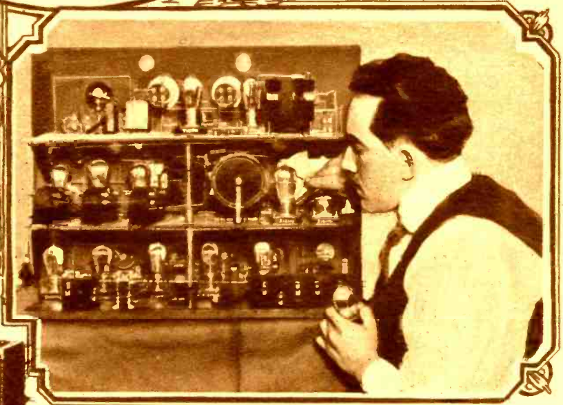
Above: This unique Super-Heterodyne was built by Henry Brinkman of Pelham, N. Y. The top shelf contains a two stage tuned radio frequency amplifier, the second shelf the detector, oscillator and intermediate radio frequency amplifiers, and the third shelf the second detector and three stages of audio frequency amplification, the third being push-pull. ©Kadel & Herbert. Left: John Shepherd, 3rd a prominent merchant of Boston owns this six tube portable radio set. It is composed of three stages of radio frequency amplification; a detector and two stages of audio frequency amplification. © International Newsreel.
