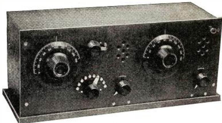
A front view of the short wave receiver. The two-point switch cuts in and out of the secondary load. Note the isolated aerial post in the upper right-hand corner of the panel.
