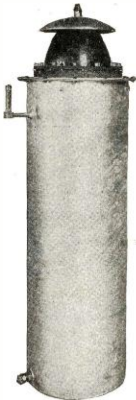
Fig. 24 This condenser built for the Navy Department to be used with a 30-K.W. arc transmitter can withstand 90,000 volts. It has a capacity of .002 M.F. and is about 5 feet high.
