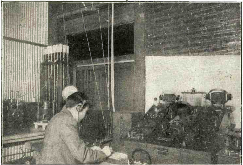
One of the old-time commercial stations that had apparatus built like a battleship, much better in fact than some of the present-day stuff. Note the two DeForest audions perched atop the left-hand receiving set. Also the large transmitting condensers in the rack by the window.
