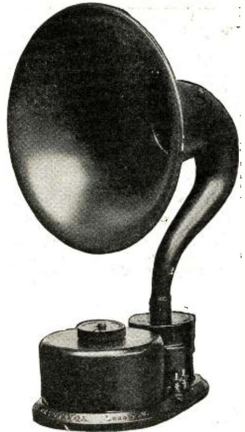
The Frenophone or crystal loudspeaker. The small phonograph motor and special headphone are situated in the casing in front of the horn.
