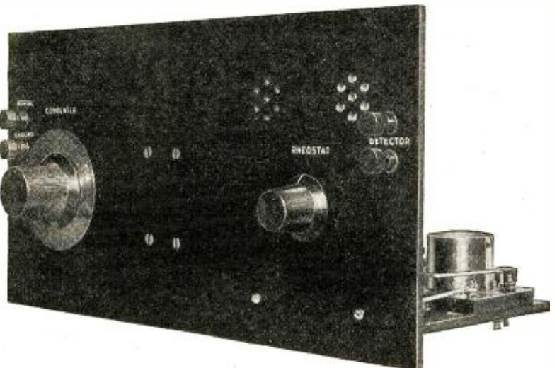
A front view of the radio frequency amplifier unit. The knob and dial on the left is the only tuning control.
