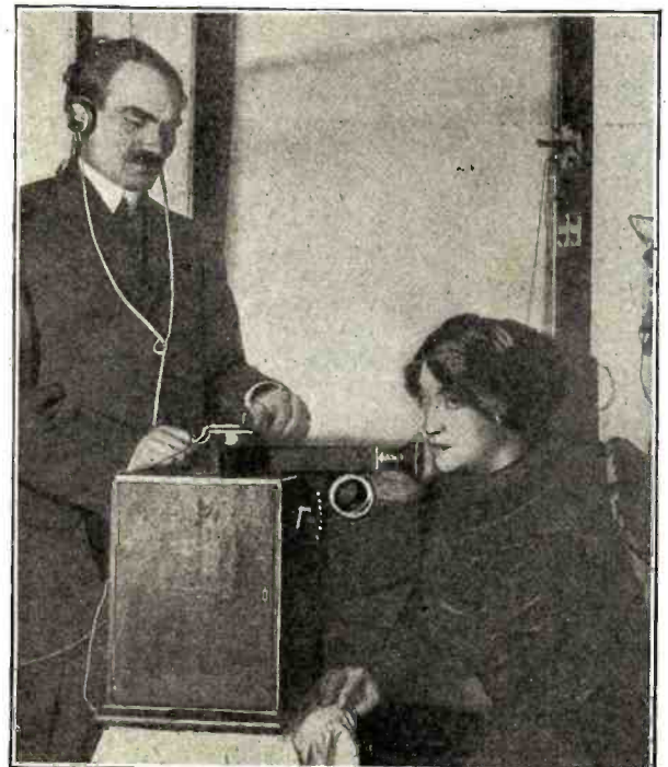
An early broadcasting station. In this picture Dr. DeForest is seen operating his arc Radiophone which could be heard in 1907 around New York; the lady is singing in the microphone.
