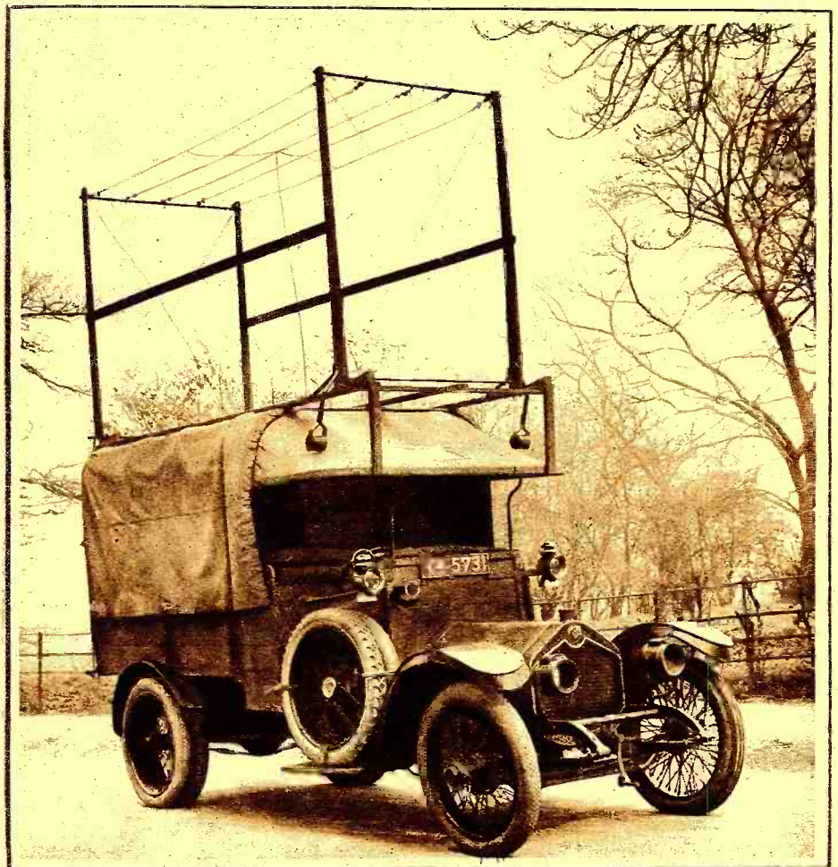
Two Views of the English Police Automobile, Showing How the Frame Supporting the Aerial May Be Folded to Pass Under Low Bridges, Trees, Etc.
