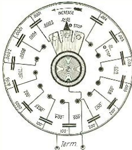
A Semi-Variable Condenser of Novel Construction. By Connecting a Low Capacity Variable Condenser Across the Main Terminals, Variation May Be Obtained Between the Successive Fixed Capacities.
