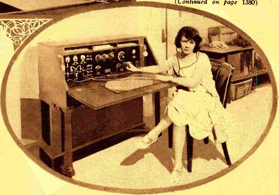
These two views of a Novel Type of Radio Desk Show How the Tuner, Amplifiers and Charging Panel are Mounted in a Stylish Cabinet. The Loud Speaker is Inside and the Horn Opens on the Side. Note the Doors of the Tone Chamber in the Lower View.
