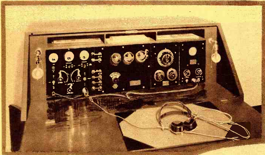
These two views of a Novel Type of Radio Desk Show How the Tuner, Amplifiers and Charging Panel are Mounted in a Stylish Cabinet. The Loud Speaker is Inside and the Horn Opens on the Side. Note the Doors of the Tone Chamber in the Lower View.
