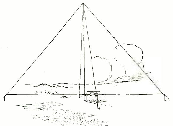
Fig. 7. Sketch Showing the Actual Appearance of the Antenna System Required to be Used With the Direction Finding Sets Described in This Article.
