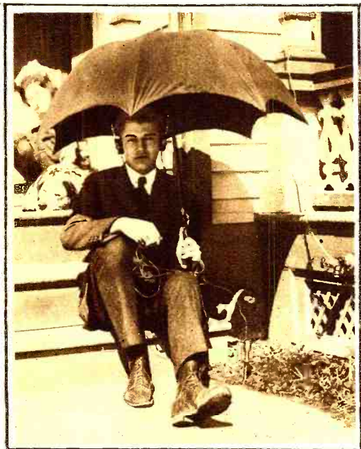
The Radio Ring in Operation. This Set is Most Efficient in Wet Weather, as a Good Ground Can be Obtained. The Umbrella Antenna is Useful in More Ways Than One.
