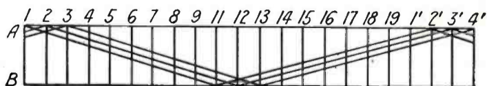
FIG. 4 Method of Winding for the Static and Rotor of a Lattice Wound Variometer.
