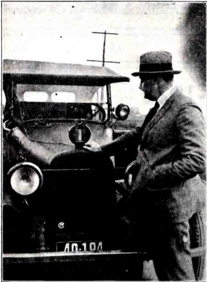
The Same as a Ship May be Guided into Port by the Guide Cable, An Automobile on the Road May be Directed by Means of the "Directometer." A Line in Which Flows a 500 Cycle Current is Installed Along the Road Inducing into a Coil Fixed on the Car Sufficient Energy to Operate an Instrument Which Shows the Driver the Correct Way to a Certain Town.
