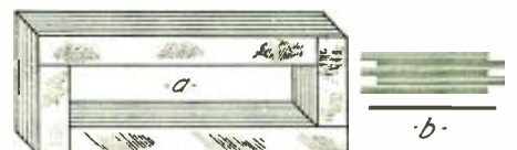
Arrangement of the Iron Core Showing How the Iron Strips Are Interleaved at Each Corner.
