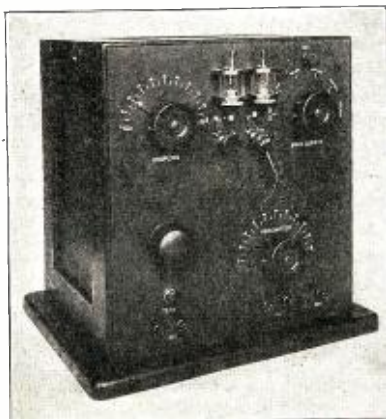
This Neat and Efficient Receiver Has a Range of From 250 to 3,000 Meters and Was Designed for Use Aboard Ships, But it May Be Used as Well by the Amateur to Receive Time Signals and Other Messages.
