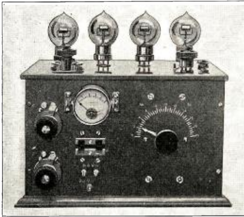
A Four-Stage Radio Frequency Amplifier Using Resistance Coupling. The Hook-up of This Apparatus is Shown in Fig. 3.
