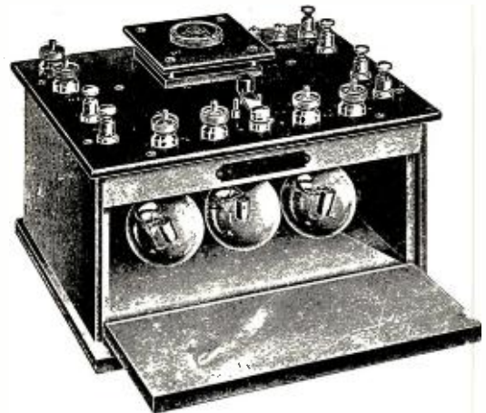
A Typical English Amplifier. Note the Compactness of this Piece of Apparatus in Which the Three Transformers and Three Tubes Are Enclosed.
