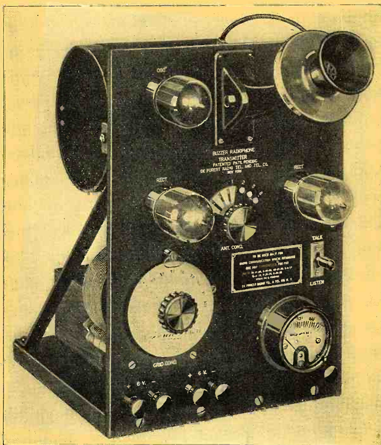
The Distinctive Feature of This Radiophone Unit Is That It Does Not Require an External Source of Plate Potential. This Solves One of the Great Problems of Low Power Radio Telephony and Thereby Opens a Wide Field of Utility for the Instrument.
