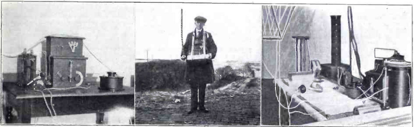
We Have Here Three Photographs of a Dutch Radio Experimenter's Activities. To the Right Is Shown a General View of the Receiving Table. The Center Photograph Is That of Mr. De Regt Receiving Messages From a Nearby Coast Station by Means of a Portable Receiving Set and a Walking Stick Aerial. To the Left Is Shown a Short Wave Receiver Capable of Tuning From 240 to 3,000 Meters.
