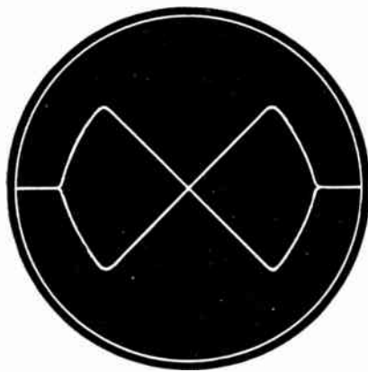
Fig. 5. Double discriminator S curve, useful for maximum amplitude adjustment of the detector
