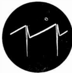
Sawtooth waveform and sync pulse of vertical sawtooth generator.
