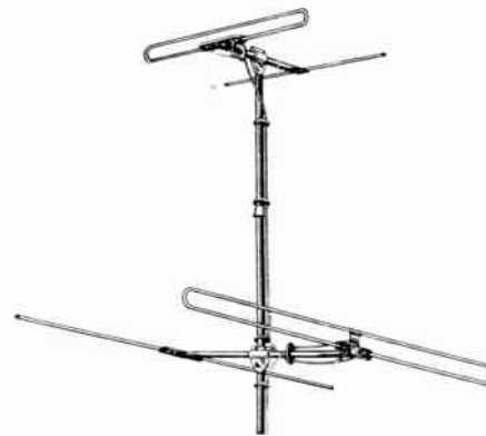
Fig. 3 A high frequency section (top) has been added in this Ward TVH-9 antenna
