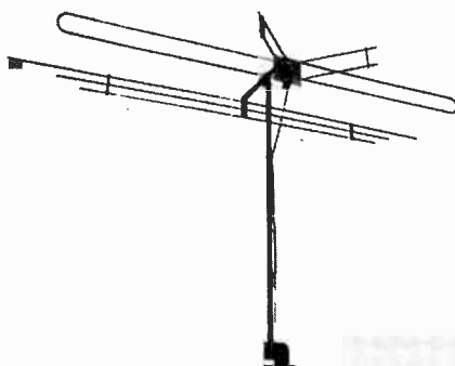
Fig. 9 2 pieces of tubing increase effective antenna diameter in this DuMont "bat wing"
