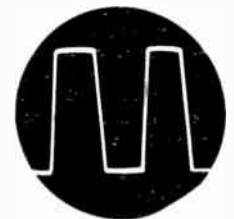
Square-wave output for measuring signal amplitude
