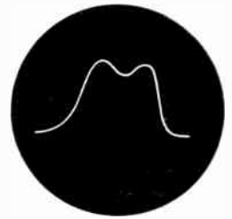
Frequency-response curve of i-f amplifier
