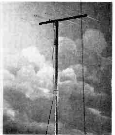
Fig. 8 The Roger Television Yagi-Beam is another fringe area multi-element antenna
