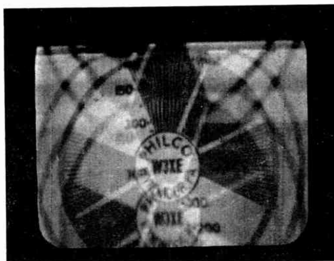
Fig. 11 Indicating that vertical hold control needs adjusting
