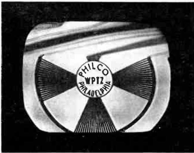
Fig. 4 Top distorted, horizontal hold control needs adjustment
