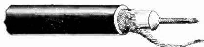
Figure 6. Simplest method of finishing up the end of a co-axial cable type of antenna lead-in.
