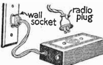
Gives clearer reception by eliminating noises caused by transformers, vacuum-cleaners, telephones, motors, etc. Keeps voltage constant, giving tubes longer life.....
