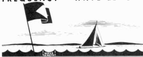
DIAGRAM 1—Radio waves are comparable to ocean waves. Wave length is the distance from crest to crest (in meters); frequency, the number of waves or cycles transmitted per second (in kilocycles or megacycles).
