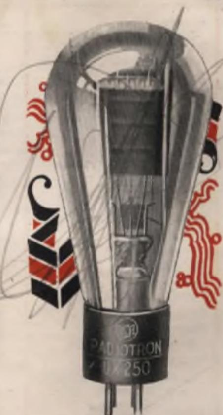
Obviously, while the new tube is capable of enormous volume it may be employed at but a fraction of its full capacity, thus securing undistorted output at all times with ample reserve power.
