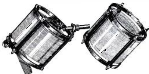
The tapped three-circuit tuner and the radio frequency coil shown will improve the operation of old style four-tube regenerative radio-frequency sets.
