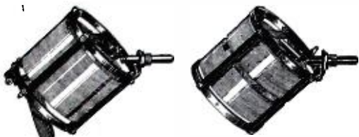
At the left is shown a low-loss three-circuit tuner. At the right is an oscillator for improving the performance of the oscillator circuit of superheterodynes.
