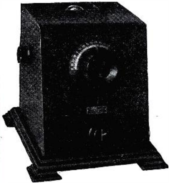
Fig. 4. An auxiliary tuned radio frequency unit which can be connected to practically any type of receiver.
