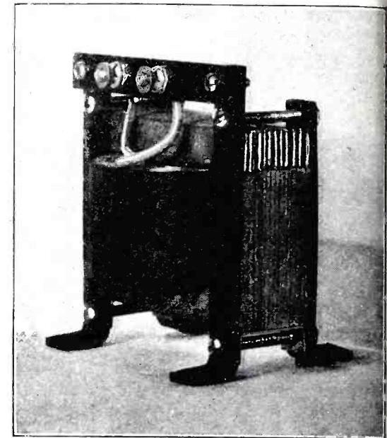
Photo by courtesy of C. E. Jacobs. A Molliformer choke coil suitable for use as an output choke between the loudspeaker and the last tube.
