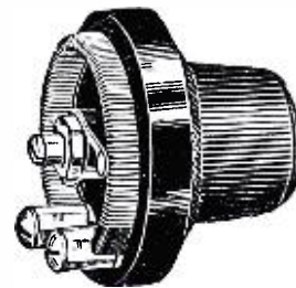
A rheostat constructed of resistance wire.
