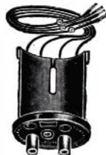
An adapter which enables the use of the UX-112 without requiring changes in wiring of set.
