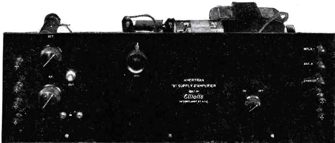
Front panel view of the "B" eliminator and power amplifier shown in the photo on this page.
