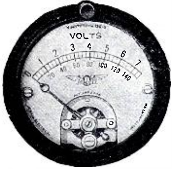
Pattern No. 135-B—Double scale, panel mounting voltmeter
