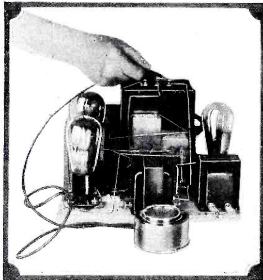
The flexible wires of a special voltmeter are touched to the output terminals of the eliminator in order to test the voltage before being encased.
