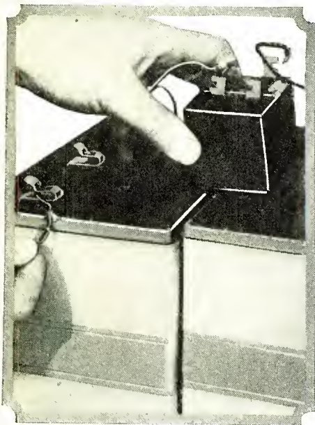
Testing the effect of various capacities across the B battery by means of condensers, as explained in the text.
