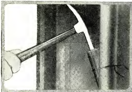
This makes a handy ground clamp.
