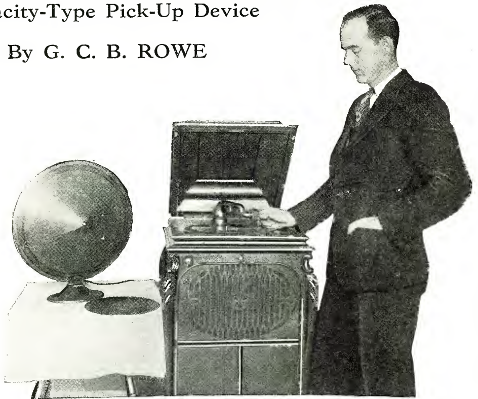
Mr. Jewell, inventor of the capacity-type pick-up device is shown playing a record, reproducing it on the loud speaker at the left.
