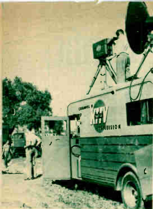
▲ JUST IN TIME FOR THE 1952 Rose Bowl classic between Illinois and Stanford Universities, KNBH came up with something new in the way of remote equipment. The "walkie-pushie" was used for the first time, and the mobile self-contained transmitter and camera moved right onto the field for close-ups. (NBC-Smith photo.)
