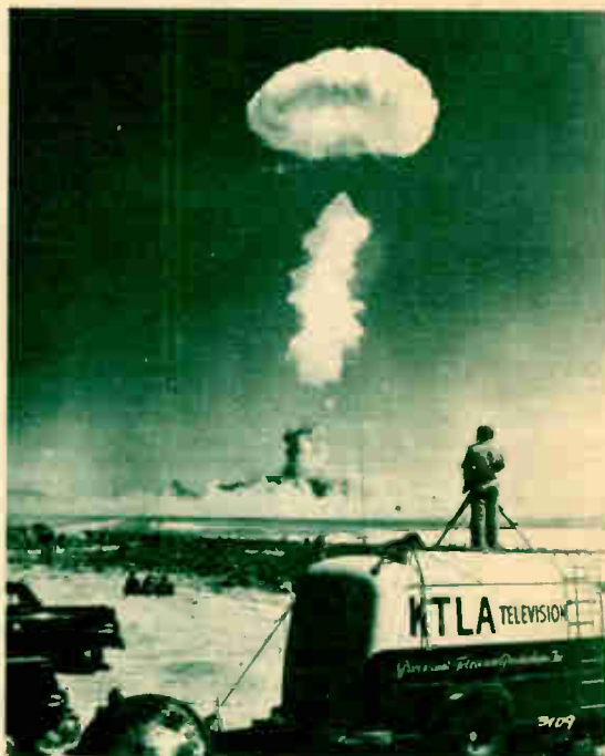
▲ THE FIRST MICROWAVE telecast of atom tests was made by KTLA's able staff. The cameras were fastened to the top of the remote truck with ropes to withstand the powerful shock of the blast.
