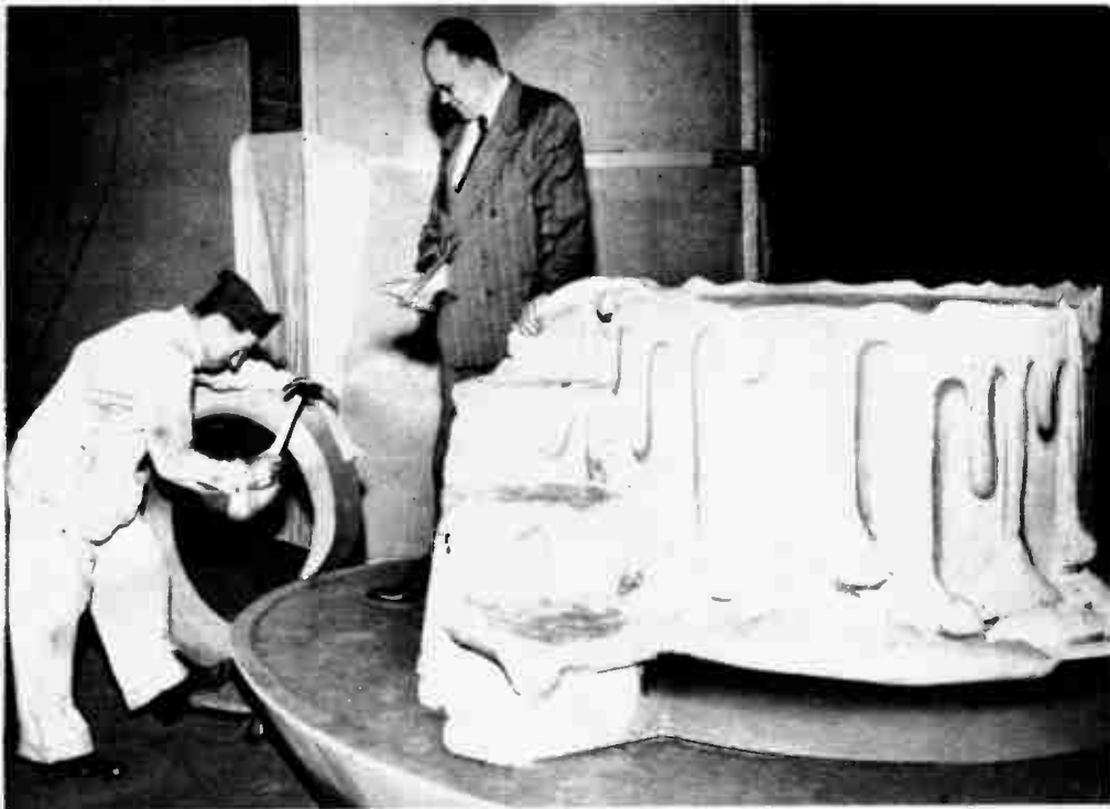
PRODUCTION MANAGER CARLTON WINCKLER SUPERINTENDS the finishing touches on the candlestick base seen on the opposite page. Plaster rendered the wooden frame solid enough to bear dancers' weights.
