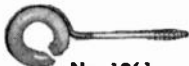
No. 1961 Split Bridle Ring Insulated Screw Eye, Overall length 3-5/8", 5/8" insulator hole, 1/4" diagonal slot.
