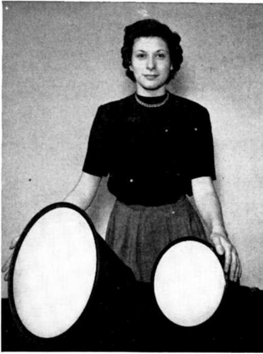
After 13 years of development, RCA's 16-inch metal kinescope, made by new glass-to-metal sealing technique, can yield a picture 2½ times larger than its smaller brother, the 10-inch tube, shown with it above.
