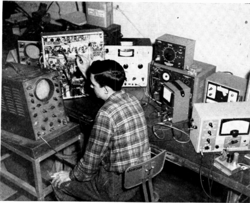
Television requires excellent service and the equipment and special technical know-how that goes with it. This man checks TV receiver's waveforms on oscilloscope.
