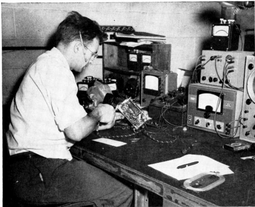
Equipped with a simple radio-type meter, a pair of pliers, a soldering iron and a mail-order catalogue the embryonic radio repairman is "in business."
