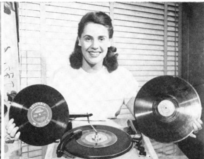
Scott Radio was first to announce a record player adaptable to all three record-playing speeds. Two pick-up arms are needed, and a brass collar slipped over the normal spindle takes care of the new RCA record.
