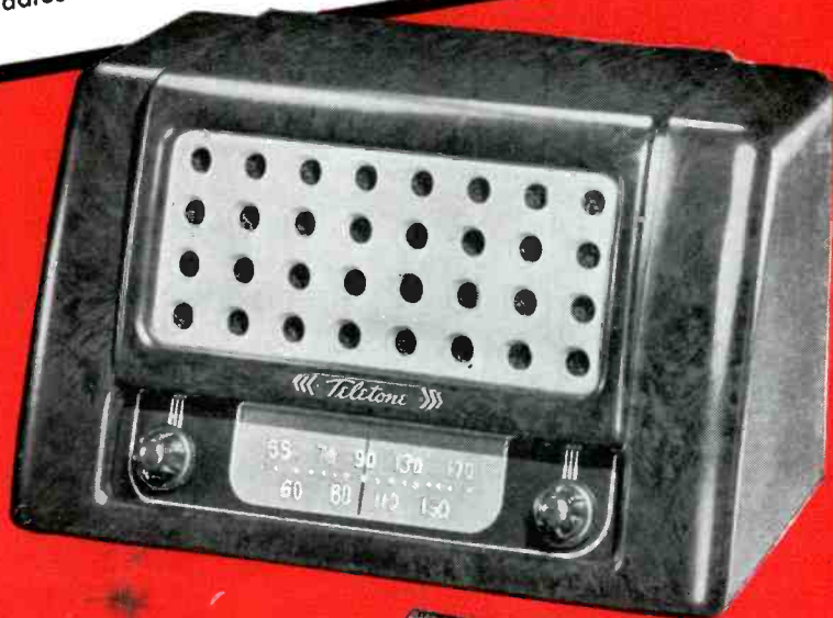
MODEL 109—Compact (AC-DC) TUTONE PLASTIC. 5" Alnico No. 5 speaker Slide rule, full-vision dial, etc.
