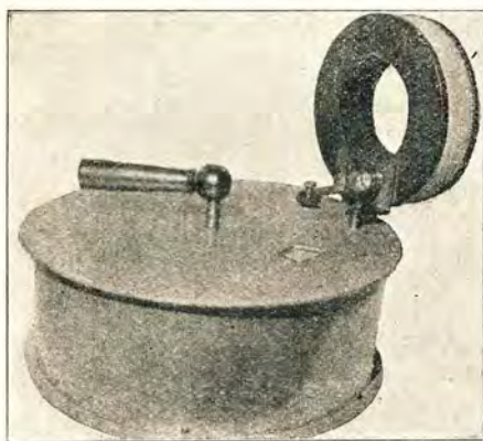
Figure No. 1—Showing arrangement of wavemeter with lamp as resonance indicator. The lamp is mounted on the side of the coil to facilitate the use of short leads. This is a very essential feature in short wave wavemeters.
