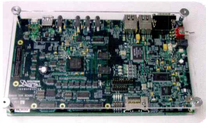
Texas Instruments chip set for Fraunhofer's MPEG Surround for audio
