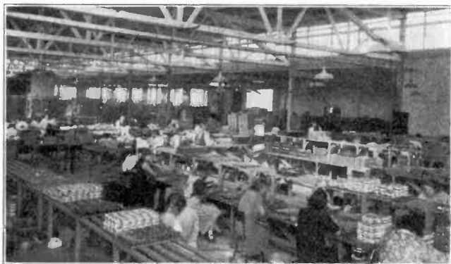
Coil winding department where the enormous number of coils are made that are required daily in the construction of Silver-Marshall Superheterodyne receivers
