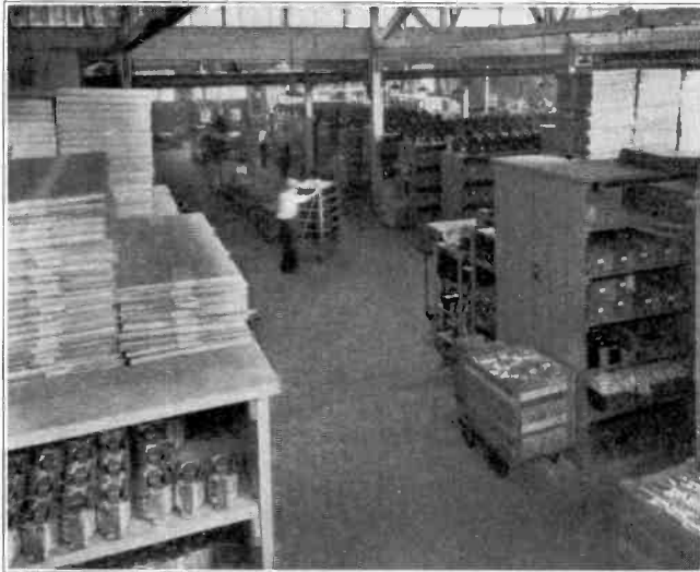
The 12,000 foot, centrally located stock-room into which all material flows and from which it is drawn as needed by the various departments. All preliminary inspections of raw materials are also made here which greatly speeds up operations in manufacturing departments
