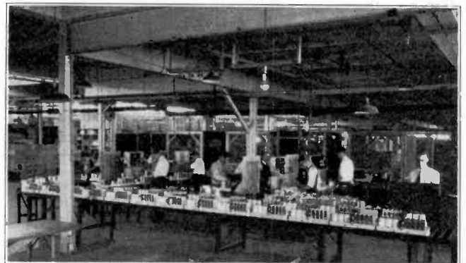
From the production lines the completed receivers go over a conveyor system through the test booths where the tuning condensers are aligned and the receivers are tested for sensitivity
