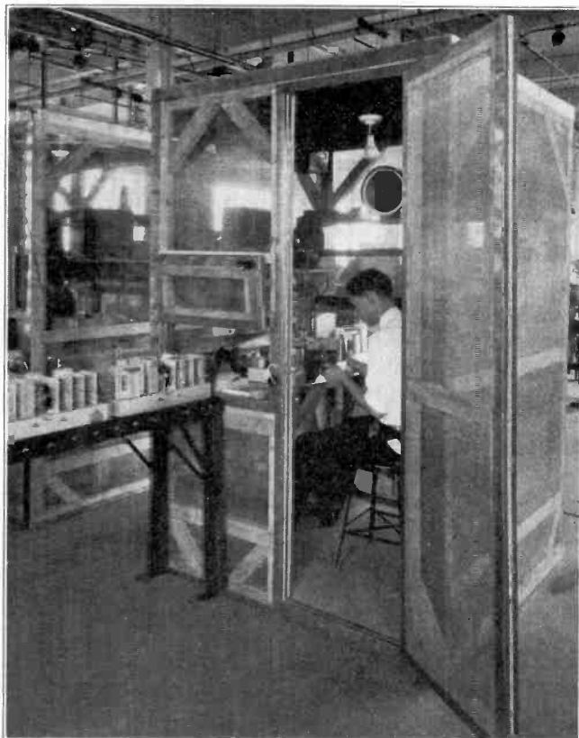
Detailed view of one of the six testing booths at the Silver-Marshall factory. The Cabinet Assembly department is the next destination of the receivers
