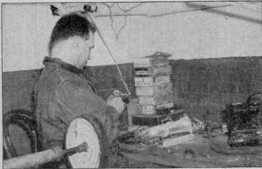
The Army Band has its own instrument repair shop, where damaged horns can be worked over. Experiments have shown that an ordinary dentist's drill is the most efficient tool for work on the delicate instruments provided Band
