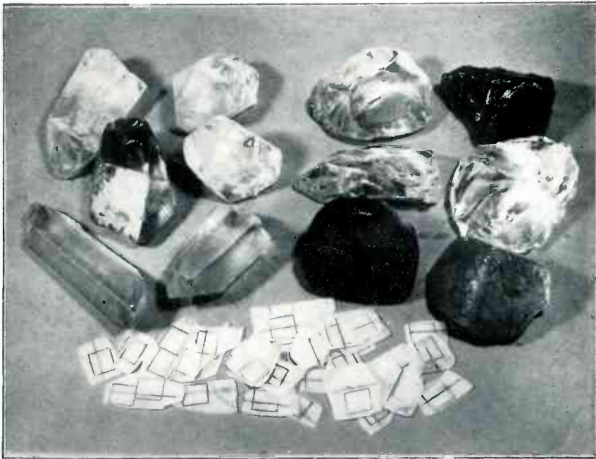
Fig. 2, Faced (left) and unfaced (right) masses of quartz of average size. The sawn wafers have 0.5 x 0.6 inch blanks marked out thereon.
