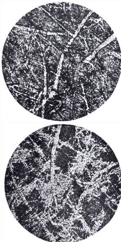
Fig. 1. Micro-photographs of condenser paper.
