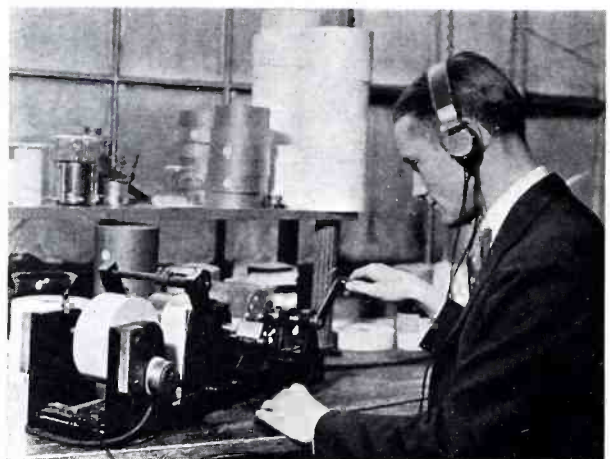
Fig. 2 (left). The porosity test. Fig. 3 (below). Conducting-particle test.
