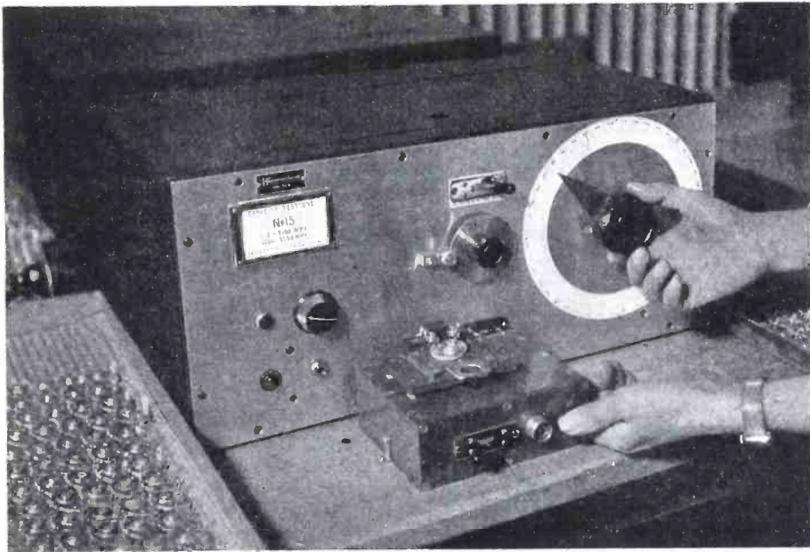
Extreme care must be taken to seat the eyelets in the Isolantite bases of trimmer condensers. These machines both insert and stake the eyelets.
