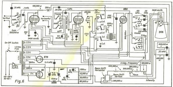
Complete schematic diagram of the portable cathode-ray oscillograph shown in Figs. 3, 4 and 5.
