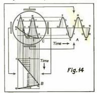
Frequency ratio 1:2 voltages A and B in phase: This shows a sine-wave voltage A applied to the vertical deflecting plates and a saw-tooth wave B applied to the horizontal deflecting plates. Wave B is linear from 0 to 14; hence, on the pattern C, the sine wave A appears undistorted. During the interval 14 to 16, the trace returns to the starting point [6.
