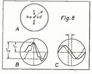
(A) Position of spot indicated by b, c, d or e would be normal (without controls) due to commercial tolerance or effect of earth's magnetic field, while a shows spot adjusted to exact center by means of the controls.
