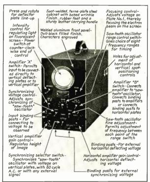
Fig. 3. External view of the portable cathode-ray oscillograph described in the text.
