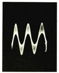
Fig. 25. A 50,000-cycle carrier modulated 50% at 400 cycles with timing axis oscillator set to 16,600 cycles.
