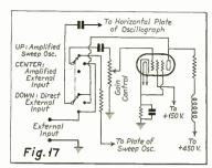
Circuit of the horizontal amplifier. Voltage gain, 75; frequency range, 20 to 90,000 cycles.
