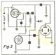
Circuit of high-pass filter, rectifier and amplifier.
