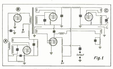
Abbreviated diagram of the oscillator unit.
