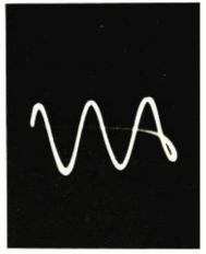
Fig. 26. A 50,000-cycle unmodulated carrier, illustrating the range of the timing axis oscillator.
