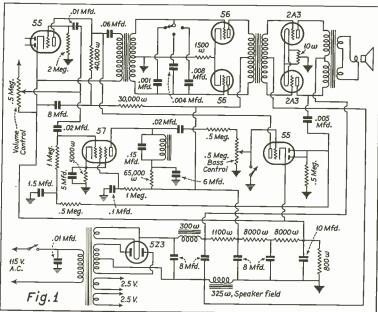
Circuit diagram of audio-frequency amplifier for a broadcast receiver, containing an automatic bass compensation system. The functions of the 57 and 55 abc tubes may be performed by a single 6F7 with slight circuit revisions.
