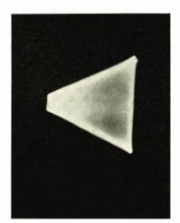
Fig. 23. Trapezoid of carrier with 75% modulation.
