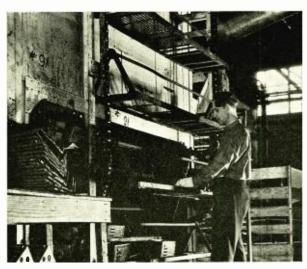
Mass drying of lacquered parts in a mechanical oven.
