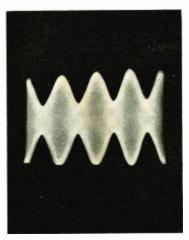
Fig. 24. A 60,000-cycle carrier modulated at 400 cycles, 50% modulation.
