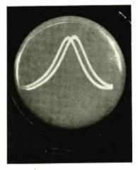
Fig. 22. The i-f curves of receiver properly aligned but off frequency.
