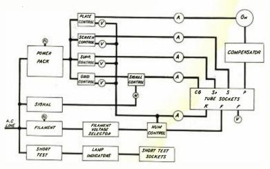
Fig. 2. Block diagram of the vacuum-tube analyzing equipment.
