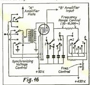
Diagram of the timing circuit. With synchronizing switch at left in upper position, synchronization from "A" amplifier; center position, synchronization from 60 cycles; lower position, synchronization externally.
