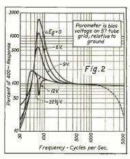
Bass control at maximum resistance load. The dotted curve is the overall response with resistance load; solid curves are of a-f amplifier only.
