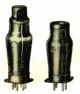
the base. The half shields are then pressed together near the top and the cap snapped on. The shoulder of the bulb acts as a pivot and the halves are forced outward at the bottom, tightening the shield in the
