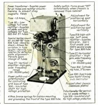
Fig. 4. Top view of the portable oscillograph chassis.
