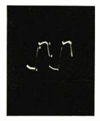
Fig. 20. Waveform of auto vibrator with unequal air gaps.
