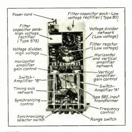
Fig. 5. Bottom view of the portable oscillograph chassis.
