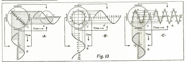
(A) Frequency ratio 1:1 voltages A and B in phase: C is the figure obtained on the screen when sine-wave voltage B is applied to the horizontal deflecting plates, and an identical voltage A is applied to the vertical deflecting plates.
