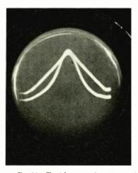
Fig. 21. The i-f curves of receiver misaligned but on frequency.
