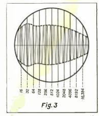
race on oscilloscope screen for an amplifier passing full a-f range.
