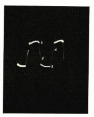
Fig. 19. Waveform of properly adjusted auto vibrator.
