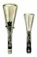
Fig. 1. The 905 and 906 cathode-ray tubes, showing comparative sizes.
