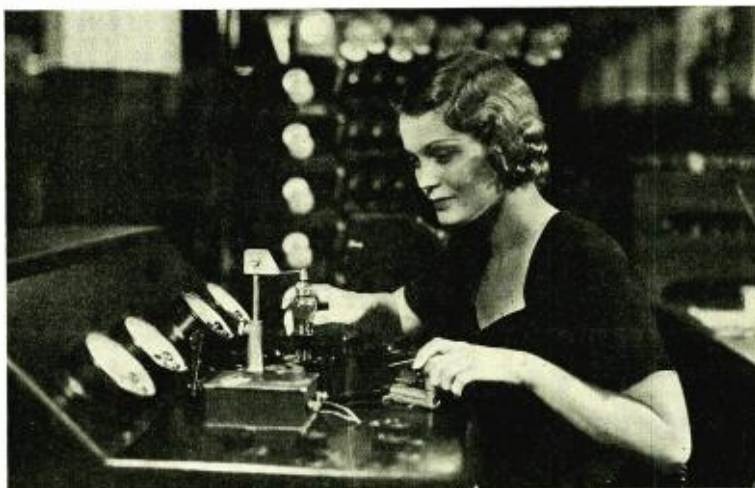
Testing tubes in factory of RCA Radiotron Division, RCA Manufacturing Company, Inc.
